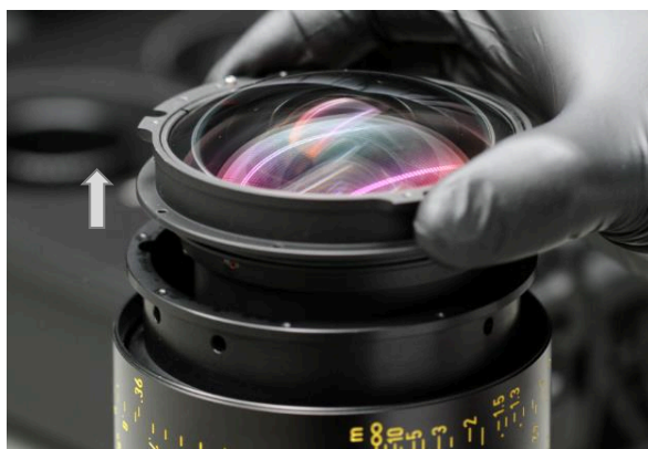
F18 front group removal by hand
