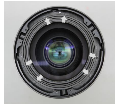
Front group screws location on F50
