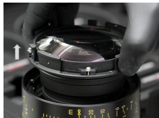
F135 front group removal by hand
