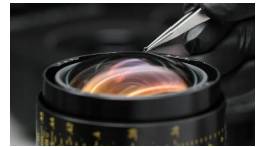
Front group screws access with and without front engraved ring
