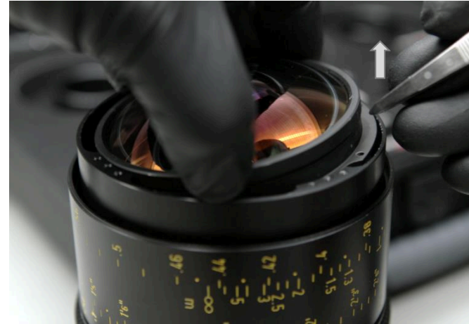
F21 front group removal with the help of a plastic head tweezers and by hand
