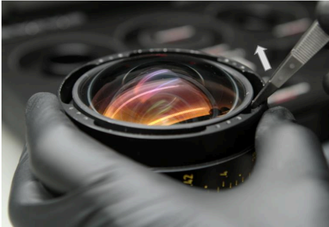
F21 front group removal with the help of a plastic head tweezers and by hand
